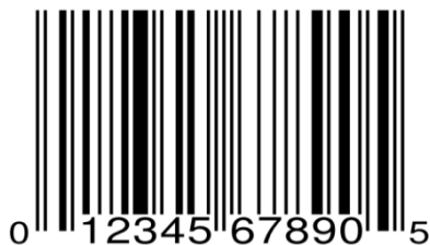
Figure 6: UPC-A barcode, encoding 12 digits
