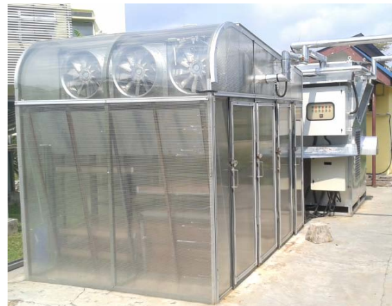
Fig. 6 Drying chamber and dryer system
