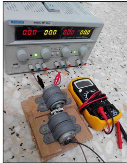
Figure. 2. 12V DC Generator with Variable DC Power Supply
