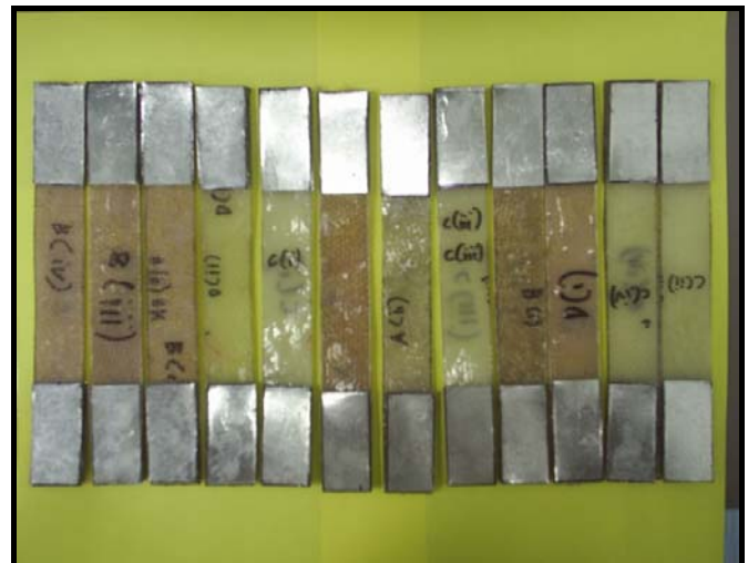
Fig. 1. Specimen for tensile test ASTM D3039
