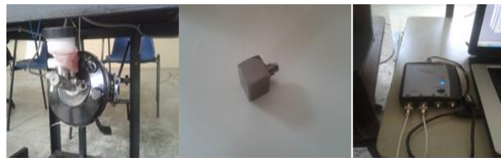
Figure 3. From left, the brake module, Dytran accelerometer and LDS Dactron portable analyzer
