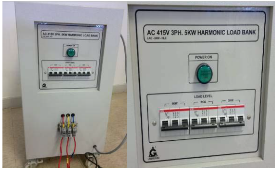
Fig. 6. Variable harmonic load bank
