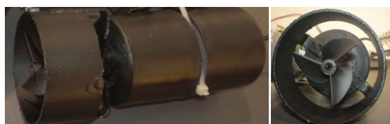
Figure 1: Completed thrusters -propeller with 3 blades
