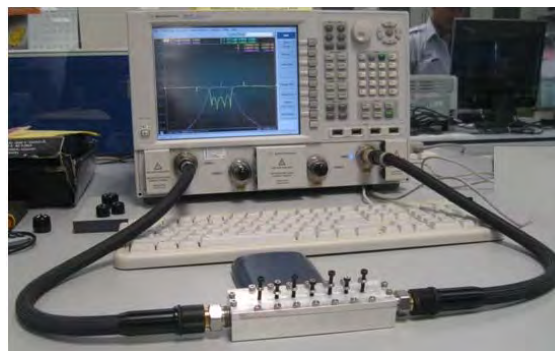
Figure 11. Measurements and Verification of the filter: (a) with lid and (b) without lid.
