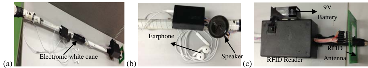
Fig. 1: Illustration of developed electronic white cane (a) Electronic white cane designed (b) Speaker and Earphone part (c) RFID reader and antenna part
