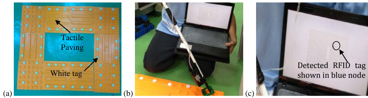
Fig. 5: Illustration of Tactile paving and RFID experiment (a) Simple map of tactile paving with planted RFID tags (b) Detect a RFID tag on tactile paving (c) Zooming in of RFID tag detected as blue node in virtual map
