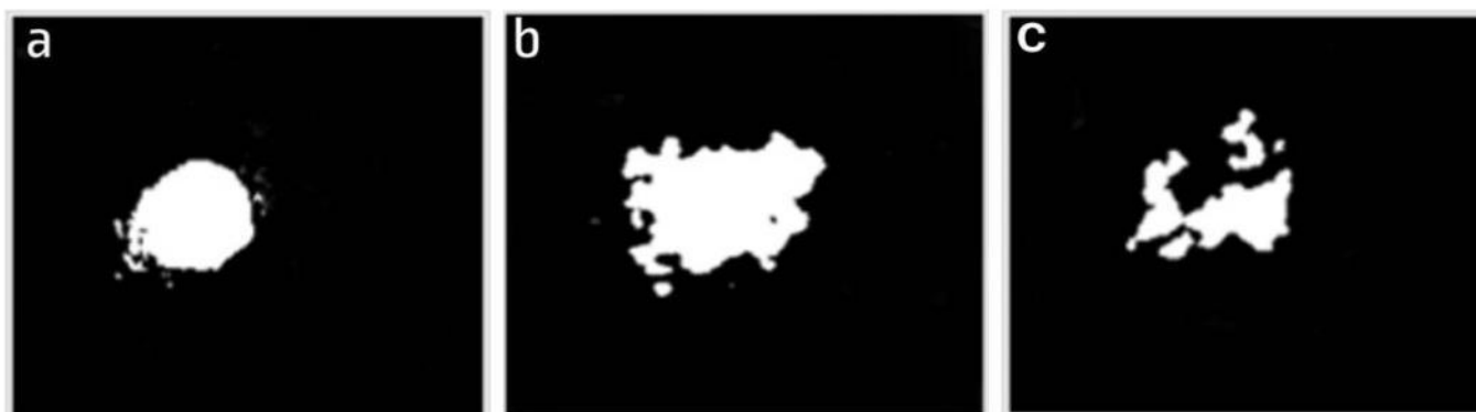
Figure 4: White and black image of chitosan based sample degradation for (a) after 1 day (b) after 14 days and (c) after 20 days. White region is fertilizer whereas black region is the agriculture soil
