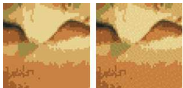
Fig. 13. The 4-bit RGB graphical image (left) and Floyd Stein-berg (right) zoomed in to 200%
