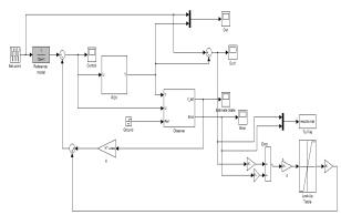
Fig. 1: Output Feedback Observer Tuning using Single Input Fuzzy Logic Controller
