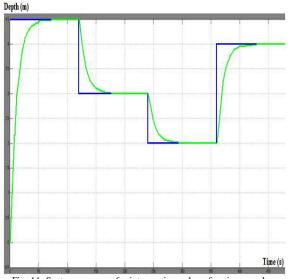
Fig. 11: System response for intersection value of optimum value tuning by BPSO
