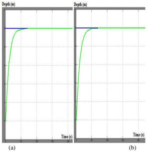
Fig. 12: System response of optimum value tuning by BPSO for (a) average value (b) intersection value.
