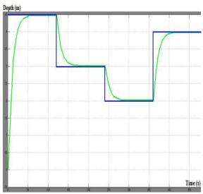
Fig. 8: System response for the average value of optimum value tuning by PSO
