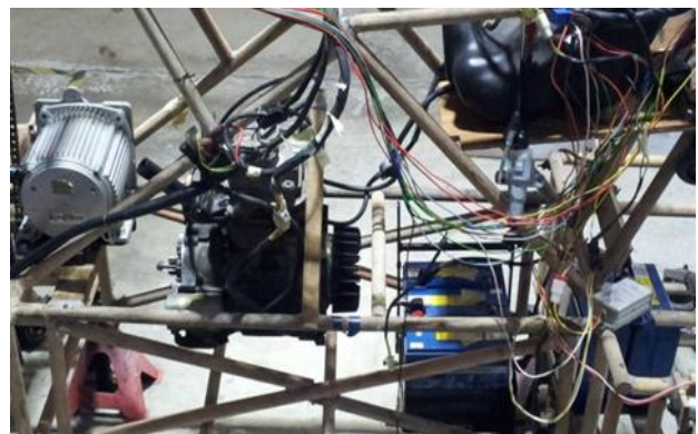
Fig. 2A. Hybrid propulsion system [12]
