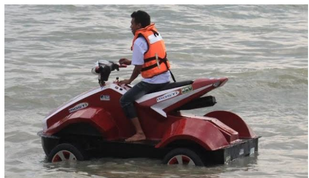
Fig. 3A. Complete AHV with hybrid propulsion system [12]
