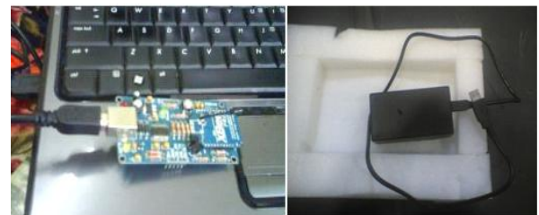
Figure 3: Connection between XBee Module and Laptop
