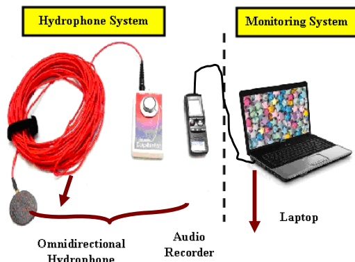
Figure 9: Hydrophone System for AUV
