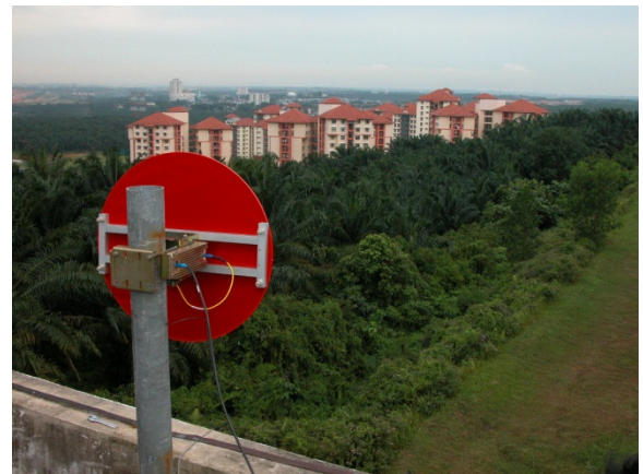
Figure 4: A trial of Point to Point Microwave Link using RLSA for FBWA application at 5.8GHz in Universiti Teknologi Malaysia
