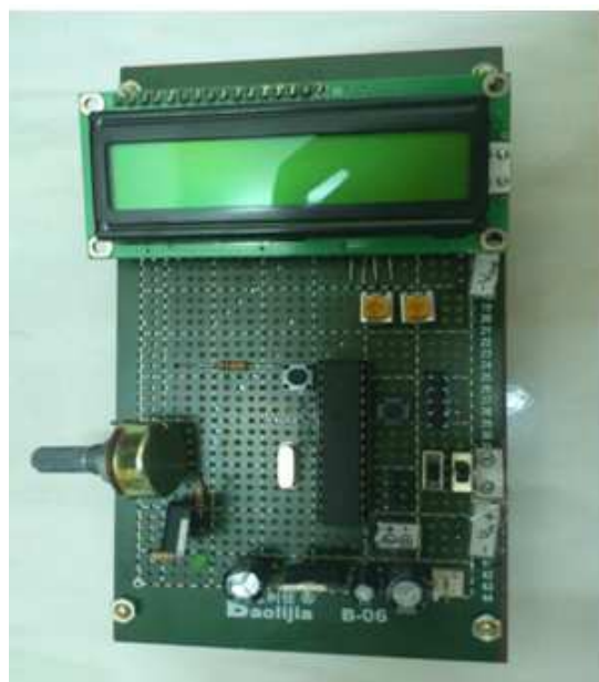
Fig. 2. The system to measure power consumption of the smartphone
