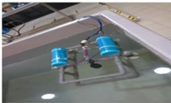
Figure 3: Portable Fish Finder attached to ROV and tested on lab pool
