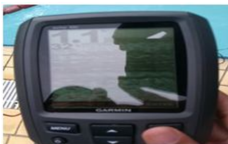
Figure 10: The device recorded 1.1m at 1.2m depth
