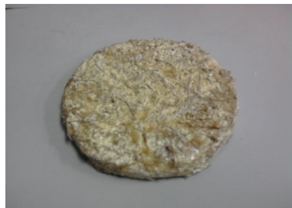
Fig. 4: The constructed sound absorber sample from the paddy straw.
