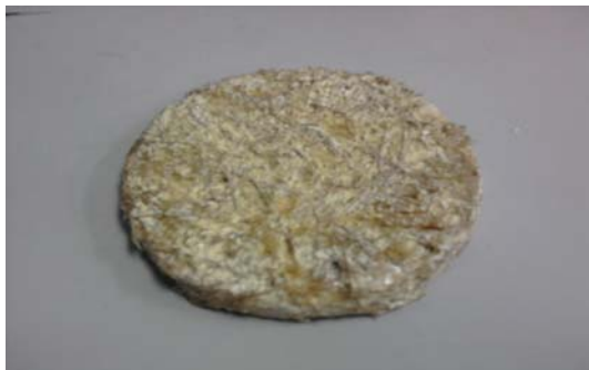
Figure 4: The constructed sound absorber sample from the paddy straw.
