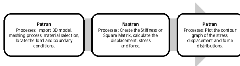
Figure 15: Process flow diagram of MSC Nastran & Patran and its FEA application.
