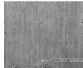
Fig. 6(b): Surfaces generated after machining under HPWAM
