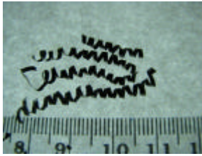
Fig. 7 (a): Chips generated under conventional coolant supply
