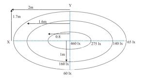
Fig. 3. Photometry lighting system of LED tube.
