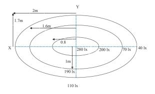
Fig. 4. Photometry lighting system of fluorescent tube
