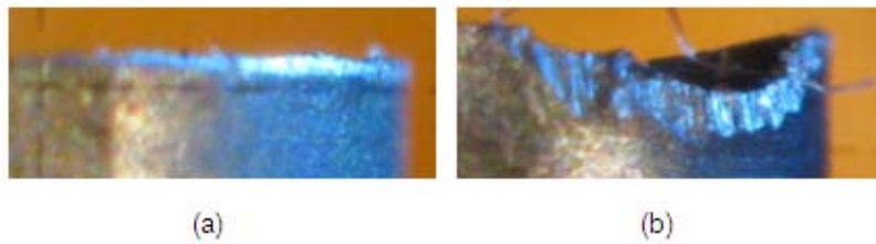
Fig. 6: Tool wear at early cutting (a) and final cutting (b) when V = 15 m/min and f = 0.02 mm/rev.
