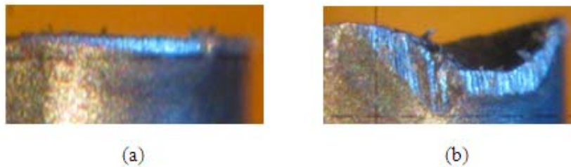
Fig. 7: Tool wear at early cutting (a) and final cutting (b) when V = 45 m/min and f = 0.04 mm/rev
