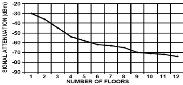
Figure 1: Signal attenuation against number of floor
