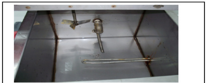
Figure 6: Inside of water bath system (Sensor, Heater and Stirrer).
