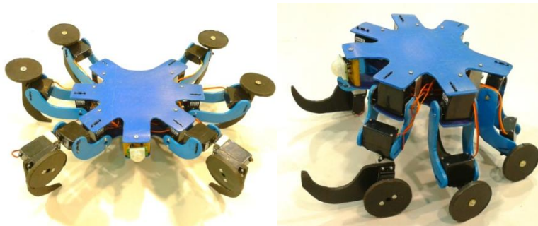
Figure 10. Hexapod Robot using Legs and Wheels
