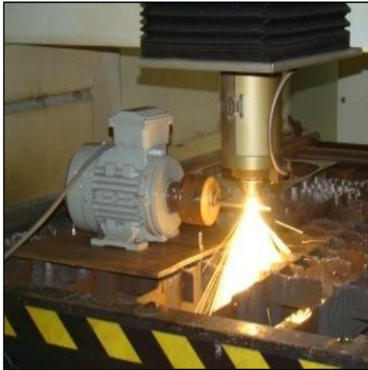
Figure 5: Laser lathing with workpiece spinning of 1500 rpm
