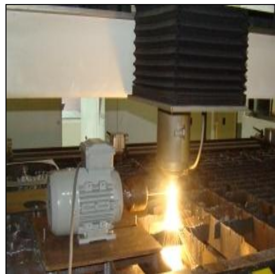
Figure 4: Laser lathing at 1000 rpm
