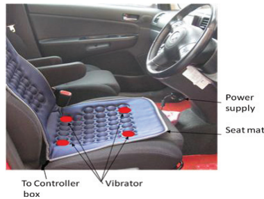
Figure 1. Developed “vibration method for Vehicle Reverse System (VRS)”
