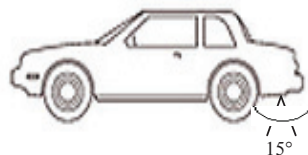
Figure 4. Directional angle for bottom sensors
