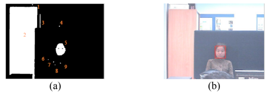
Figure 3. Morphological processing and connected region analysis. (a) Image after morphological processing. (b) Region of interest
