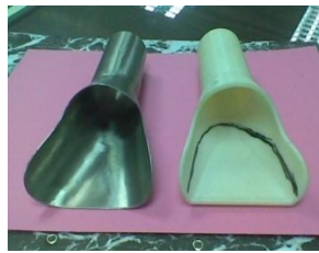
Figure 10.0b Scoop from Vendor and Rapid Prototyping
