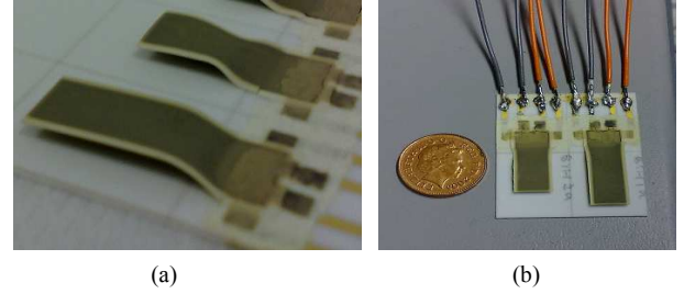
Fig. 2. (a) Fabricated samples and (b) Samples connected to terminals ready for polarization.
