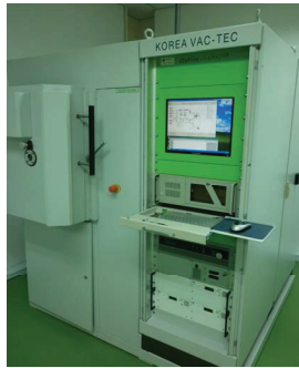
Figure 1. PVD unbalanced magnetron sputtering system VACTEC Korea model VTC PVD 1000.
