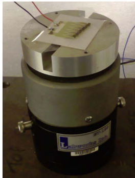
Fig. 3 Device under test on a vibration generator
