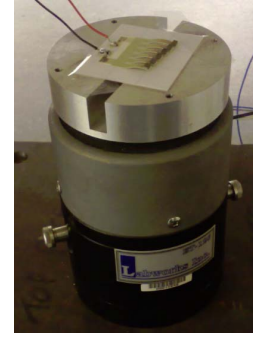
Fig. 7 Device under test on a vibration generator
