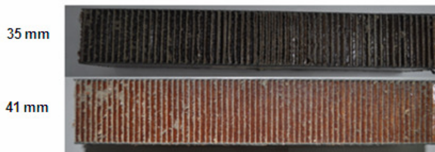
Fig. 1. Sample of the paper honeycomb sandwich panel with thickness of 35 mm and 41 mm.
