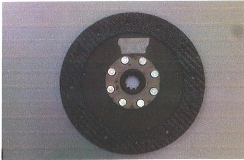
Fig. 8. Carbon composite clutch facing is riveted to cushion disc and spline hub
