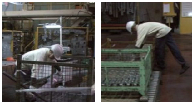
Figure 1. Workers arrange the metal stamped parts in standing position and awkward working posture
