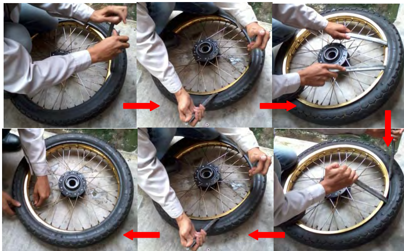
Fig. 2 Current practice of the motorcycle tire dismounting process
