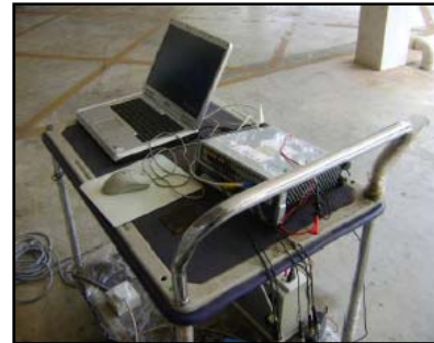
Fig. 5 Experiment setup for Operational Deflection Shape (ODS)
