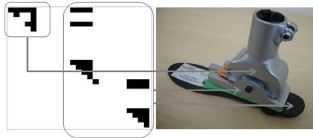
Figure 10: The laboratory prototype PF design that was constructed based on the proposed numerical profile.
