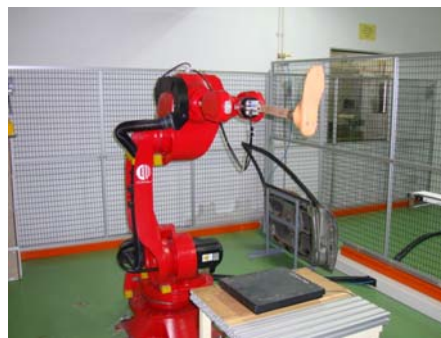
Figure 11: Above is an adaptation of an industrial robot to simulate an amputee's stance phase. Although the accuracy of this approach may be questionable it did provide a means through which the prototype FAM could be tested without the need for the involvement of an amputee.
