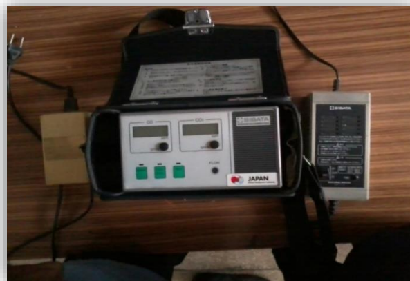
Figure 3. SIBATA CO 2 meter
