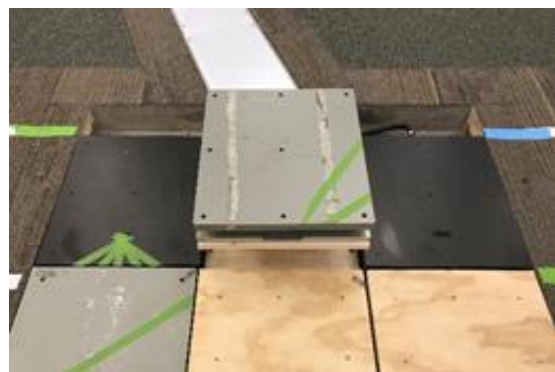
Figure 1. Force platform setup used for data collection, containing 3 AMTI force platforms, with one for platform built into a step.
