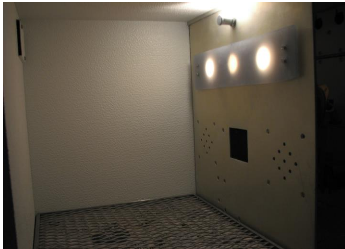
Figure 1. Interior view of experimental chamber, showing houselight, keylights, and feeder opening.
