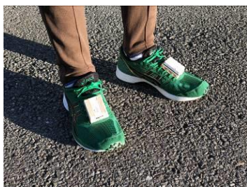
Figure 1: IMU sensors on shoes
