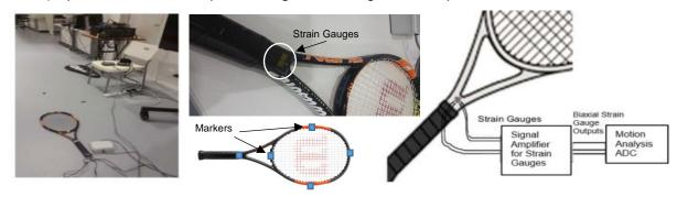
Figure 2: Strain Gauge on Tennis Racket Set-up
