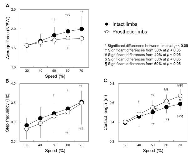
Figure 1: (A) average vertical ground reaction force (F<sub>avg</sub>), (B) step frequency (Freq<sub>step</sub>), and (C) contact length (L<sub>c</sub>) of intact limb (black circles) and prosthetic limb (white circles) across five running speeds. Error bars represent a standard deviation.
