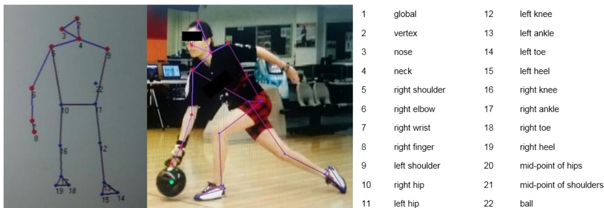
Figure 1: Digitized landmarks for the calculation of 3D bowling biomechanics
