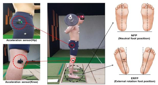
Figure 1: Attachment position of acceleration sensor and definition of foot position.
