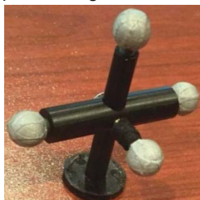
Figure 1. Plastic rod reflective marker cluster for trunk kinematics.
